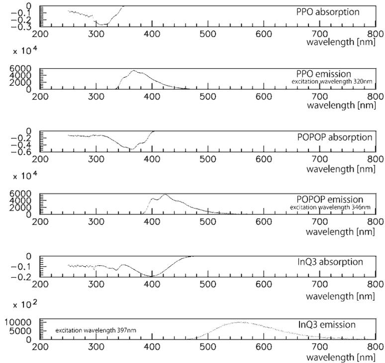
Figure 4. Absorption and emission of PPO, POPOP and InQ<sub>3</sub> in PhCN.
