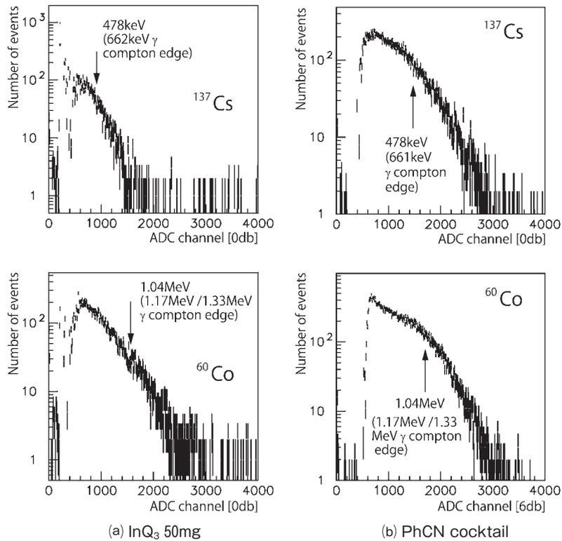
Figure 8. Observed spectrum of  $\gamma$ 's via SC-48 lter. (a) The light yield was lost about 34% in case of PhCN cocktail scintillator containing  $\text{InQ}_3$  complex. On the other hands, (b) 23% of the light yield of PhCN cocktail scintillator still remained via SC-48 lter.
