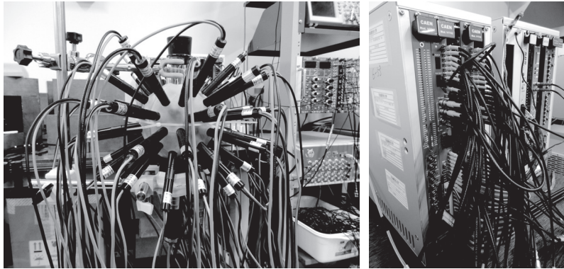
Figure 2. Photographs of UNI-ZICOS detector and CAEN V1742 digitizer.
