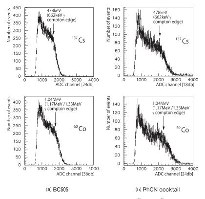
Figure 6. Photon spectrum of electrons emitted by γ's interaction using <sup>196</sup>Cs and <sup>60</sup>Co sources for both standard liquid scintillator BC505 and PhCN cocktail scintillator.
