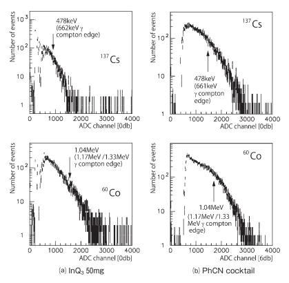
Figure 8. Observed spectrum of  $\gamma$ 's via SC-48 lter. (a) The light yield was lost about 34% in case of PhCN cocktail scintillator containing  $lnQ_3$  complex. On the other hands, (b) 23% of the light yield of PhCN cocktail scintillator still remained via SC-48 lter.
