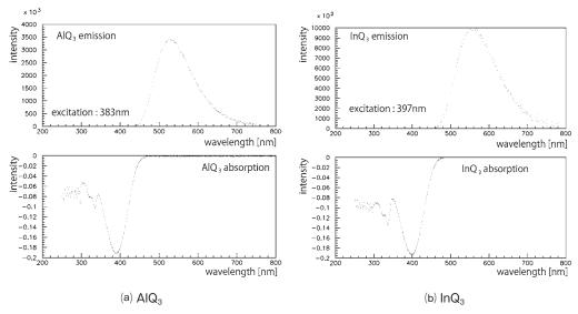
Figure 3. Photo luminescence and absorbance of (a) AIQ<sub>3</sub> and (b) InQ<sub>3</sub> complex dissolved in PhCN are shown. The maximum emission wavelength of AIQ<sub>3</sub> and InQ<sub>3</sub> were found at 529.9nm and 559.3nm with the excitation wavelength at 383nm and 397nm, respectively. Also the maximum absorption wavelength were located at 389.6nm and 394.7nm, respectively.
