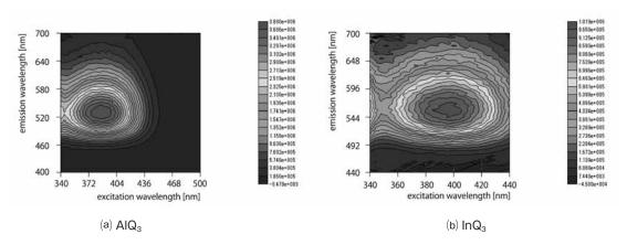
Figure 2. 2-dimensional plot of uorescence of (a) AIQ<sub>3</sub> and (b) InQ<sub>3</sub> complex dissolved in PhCN are shown. Horizontal and vertical axis shows the wavelength of excitation and emission light.
