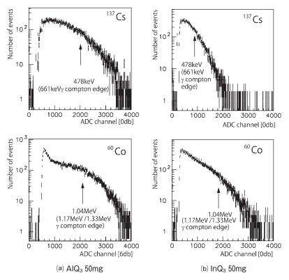
Figure 7. Observed energy spectrum of (a)  $AIQ_3$  50 mg (b)  $InQ_3$  50 mg dissolved in PhCN cocktail scintillator for  $\gamma$ 's from  $^{136}Cs$  and  $^{60}Co$ .
