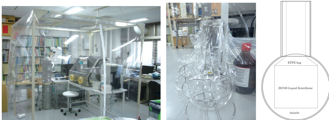
Figure 5. The left panel shows a clean booth and the grove box. The middle panel shows the specially made round bottom flask using the ultra-pure quartz. The chimney could be used for PMT guide. The right panel shows the figure of the inner cubic bag which has 10 cm in one side
