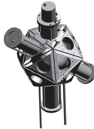
Figure 2. The left side panel shows the designed 2 \nu -ZICOS detector. The ultra-pure quartz round bottom flask and 20 Hamamatsu H3378-50 photomultipliers will be used for the observation of scintillation lights. The right side panel shows a sample of the PMT mounting jig.
